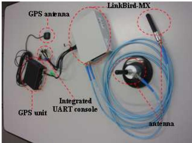
**Figure4:LinkBird-MX Configuration Image**
